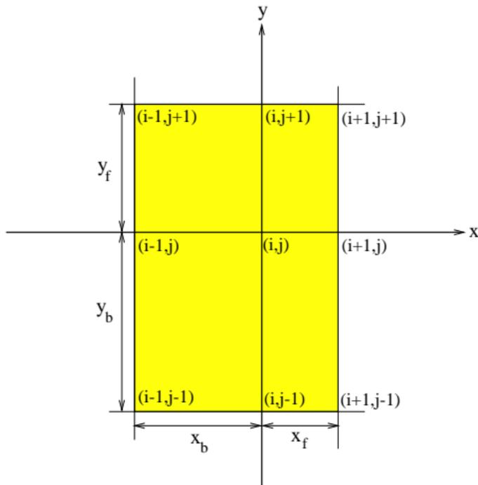
Figure: The stencil used for the steady  $\psi$ - $v$  formulation.
