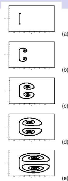
**Figure:** Streaklines for  $Re = 400$  at (a)  $t = 1$ , (b)  $t = 2$ , (c)  $t = 3$  (d)  $t = 4$  and (e)  $t = 5$ .
