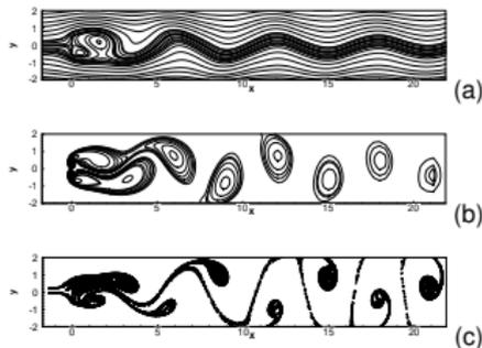
**Figure:** For  $Re = 40$ : (a) the streamlines, (b) the vorticity contours and (c) the streaklines behind the flat plate depicting vortex shedding.
