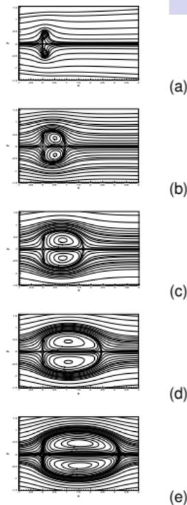
**Figure:** Streamlines for  $Re = 400$  at (a)  $t = 1$ , (b)  $t = 2$ , (c)  $t = 3$  (d)  $t = 4$  and (e)  $t = 5$ .
