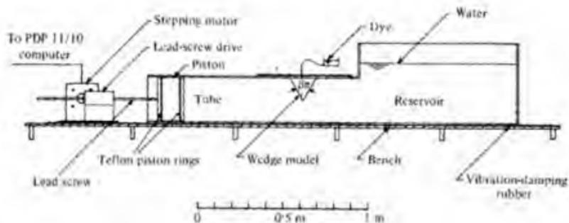
**Figure:** Experimental set-up for starting vortex flow visualization by Pullin and Perry ([13]).
