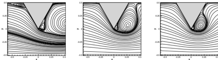
**Figure:** Streamlines for accelerated flow past a  $60^\circ$  wedge at time  $t = 0.8$  for  $Re = 1560$  (left,  $m=0$ ),  $Re = 6621$  (middle,  $m=0.45$ ) and  $Re = 6873$  (right,  $m=0.88$ ).
