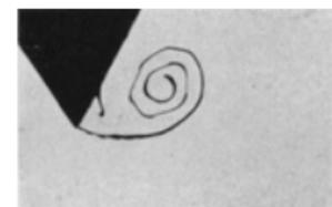
Figure: Streaklines for  $Re = 6873$  at (a)  $t = 2.8$ , (b)  $t = 4$  and (d)  $t = 5$  (Present).
