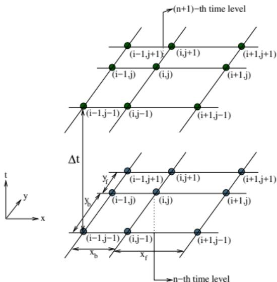
Figure: The stencil used for the unsteady  $\psi$ - $v$  formulation.
