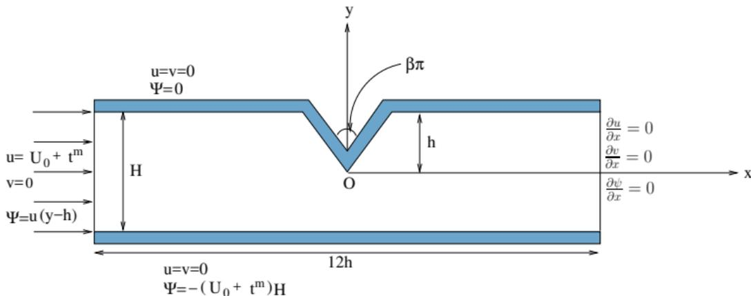
Figure: Configuration of the flow past a wedge in accelerated flow problem ([8, 9, 13, 14]).
