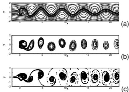
**Figure:** For  $Re = 100$ : (a) the streamlines, (b) the vorticity contours and (c) the streaklines behind the flat plate depicting vortex shedding.
