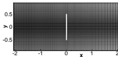
Figure: A typical  $301 \times 101$  grid (top) and Close up view of the grid near the surface of the plate (bottom).
