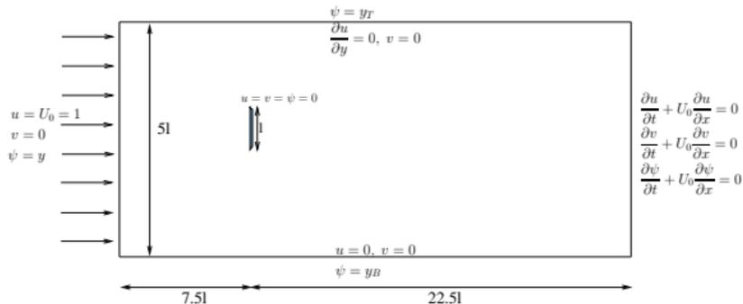
Figure: Configuration of the flow past a flat plate in uniform flow problem ([10, 11, 12]).
