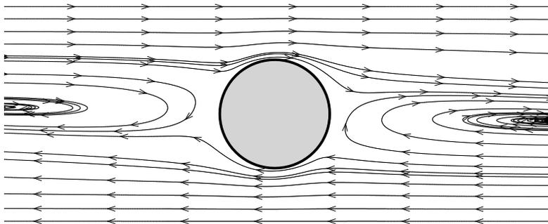
**Flow field around a freely rotating sphere in simple shear flow at  $Re=50$ .**
