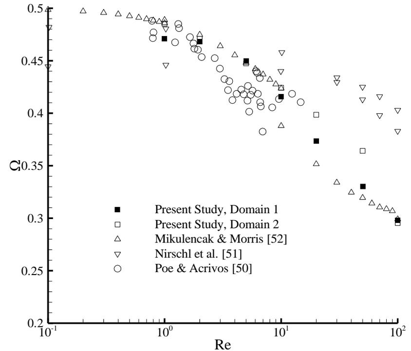
**Rotation rates of freely suspended spheres in a simple shear flow.**
