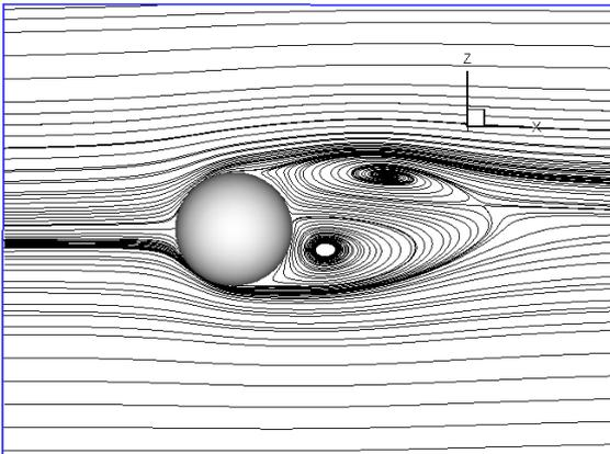
**Re=250: Quasi-steady non-axisymmetric flow with tilted vortex wake. In transition region between 210 – 270 (from steady axisymmetric to unsteady shedding).**
