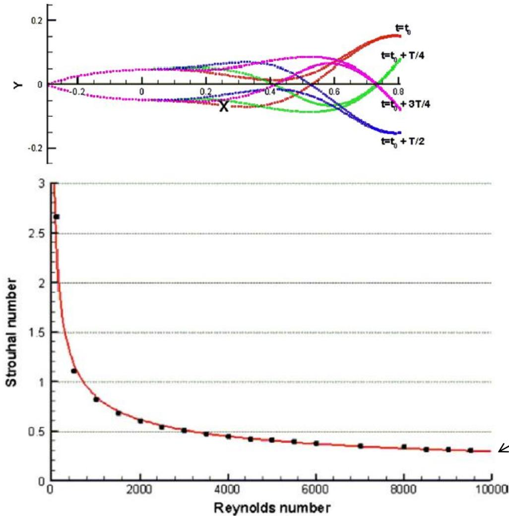
Fig. 21. Strouhal number  $St$  versus Reynolds number  $Re_f$  for steady swimming of the simulated fish.
