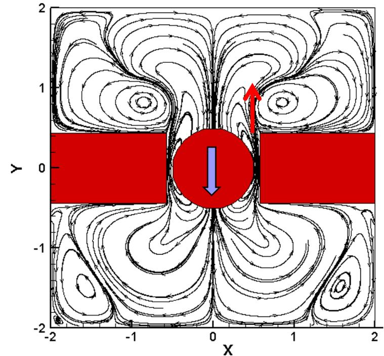
Oscillating cylinder in a narrow slot. Gap=0.075D.
