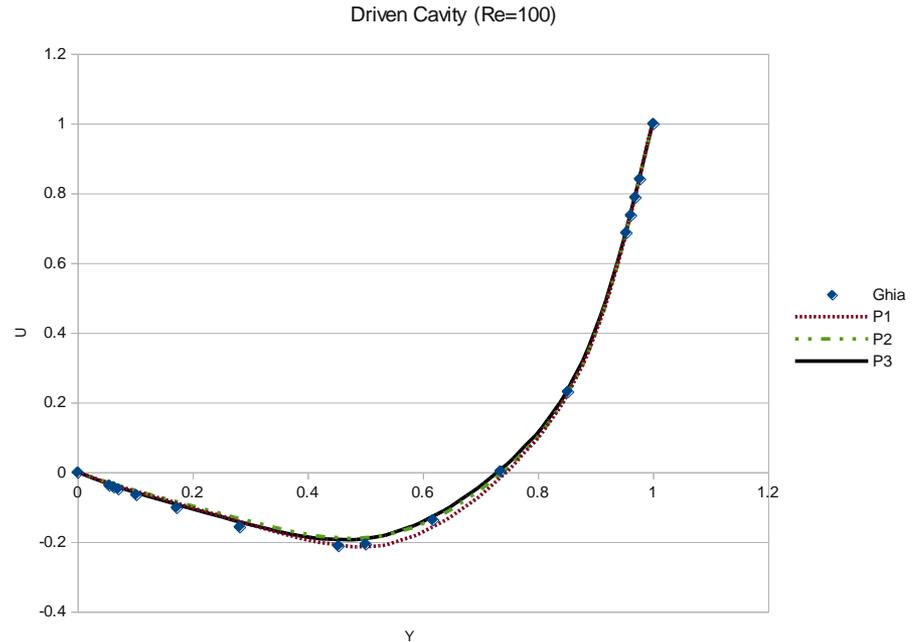
**U-velocity along  $x=0.5$ . Meshfree solution with 848 grid nodes versus Ghia et al. ( $129^2 = 16,641$  nodes).**
