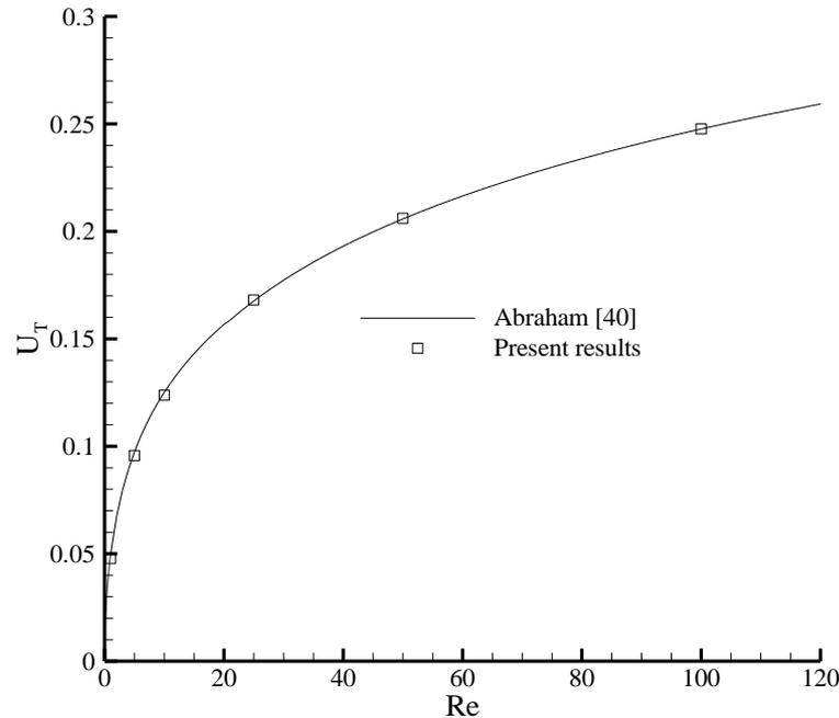
**Comparison of terminal velocity of a free falling sphere at different Re.**
