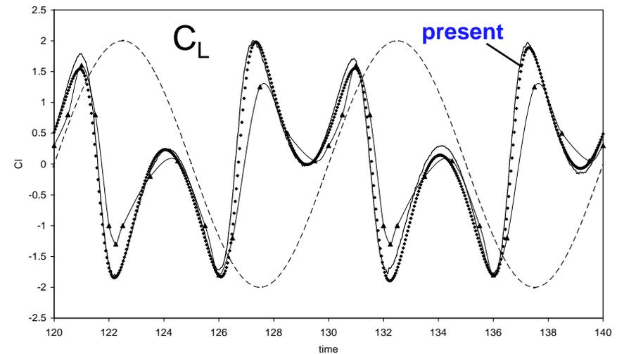
$C_D$  and  $C_L$  for longitudinally oscillating cylinder at  $Re=200$  and  $KC=U_{max} T/D=10$ .
