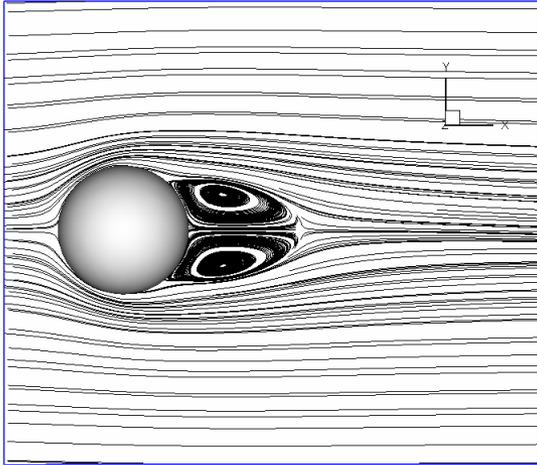
**Re=100: Steady axisymmetric flow with attached vortex.**
