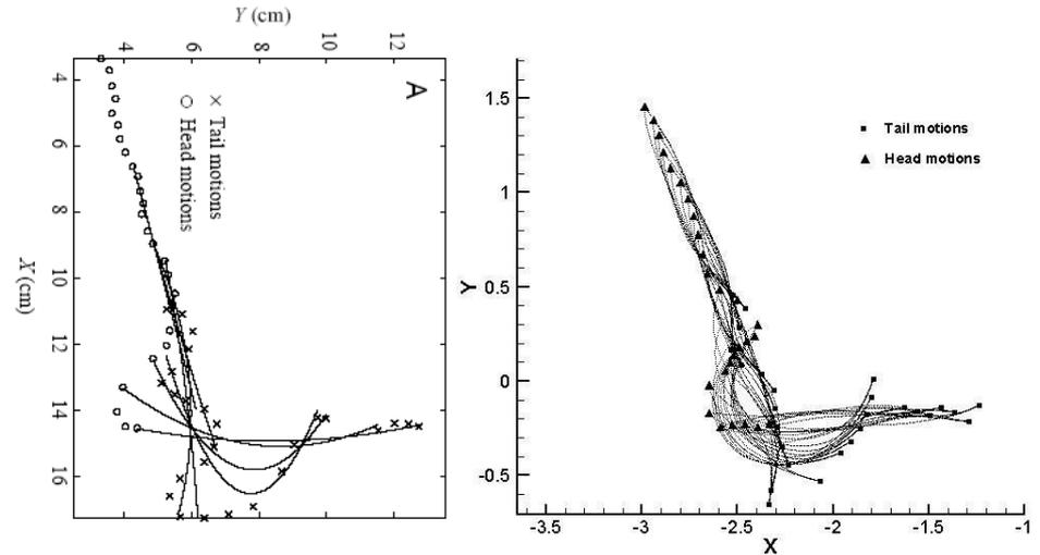
Trajectory of fish turning: (left) live fish from Wolfgang et al. [36] turning through 72-75 deg., (right) present simulation of fish turning through 70 deg. at  $Re_f = 2000$ .
