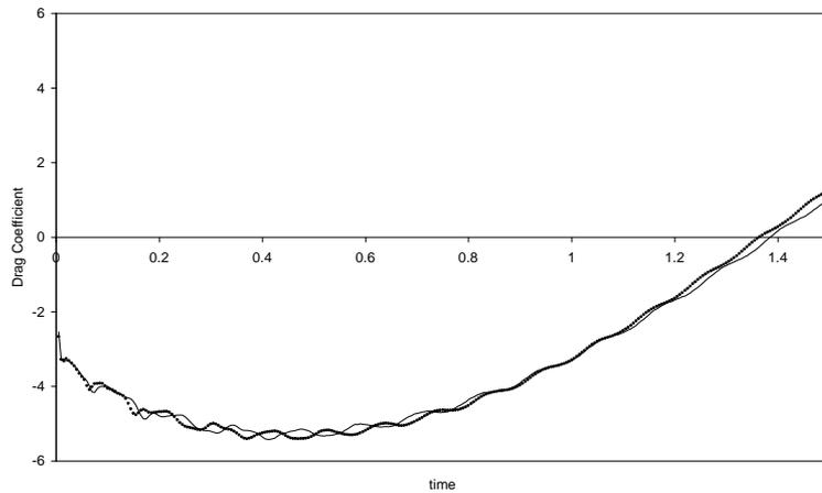
Drag on Sinusoidally started cylinder at  $Re=20$ .
