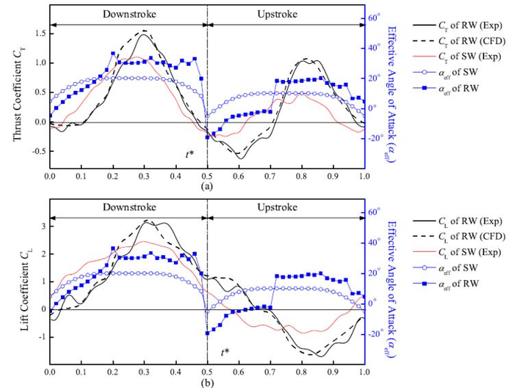
Figure 6.8: Experimentally and numerically obtained transient thrust and lift coefficients ( $C_T$  and  $C_L$ ) of the rear wing in the case of in-phase stroking ( $\varphi = 0^\circ$ ). The effective angles of attack ( $\alpha_{\text{eff}}$ ) of the rear wing and the single wing are also included.
