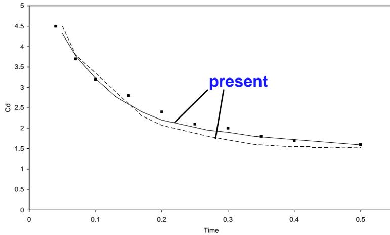
Drag on Impulsively started cylinder at  $Re=100$ . ALS-GFD case:  $u \rightarrow 1.0$  in time 0.02.
