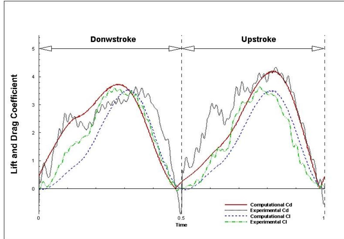
Comparison for lift and drag for fruit fly type wing at  $Re = 150$ .
